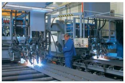
Before the next processing stage, web plates are welded into place to protect the girder against twisting; stiffeners are inserted to improve the overall stability of the structure. Following assembly on the box girder line, the box girder is ready for processing by the portal welding unit.
