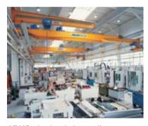
ABUS single girder wall travelling cranes are installed on a separate track below other types of travelling crane. They are the ideal solution for serving several working areas at the same time. The ABUS EKL single girder wall travelling crane is designed for spans up to 12 m and load capacities up to 5 tonnes.
