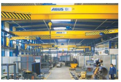
ABUS two fall wire rope hoists are designed for high lifting speeds and load capacities up to 20 t. In this example, wall-mounted jib cranes provide flexible material handling on the lower level.
