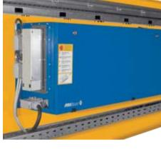
The **ABULiner** is an effective solution when precise positioning is required with variable speed hoists. This frequency converter also allows the maximum speed to be increased above the rated speed when lifting part/reduced loads. ABULiners are also available for crane and trolley travel.
