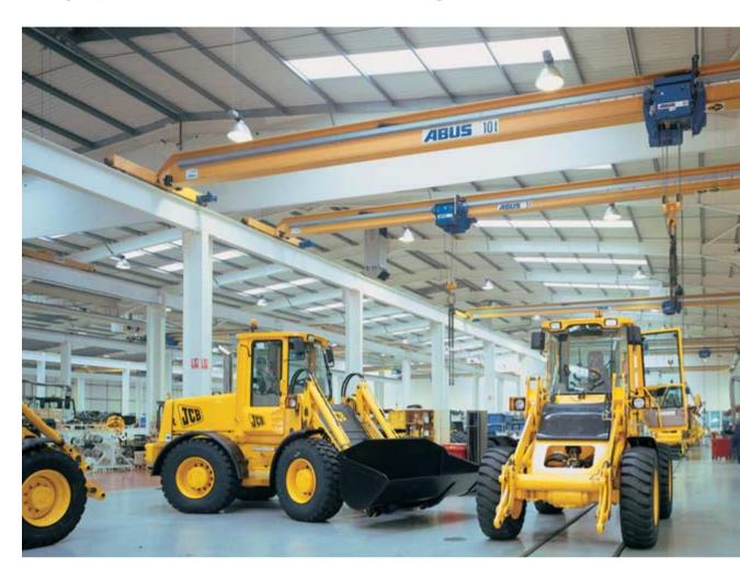
ABUS single girder travelling cranes allow efficient material handling with load capacities up to 16 t and spans up to 39 m even in halls with low ceilings.
