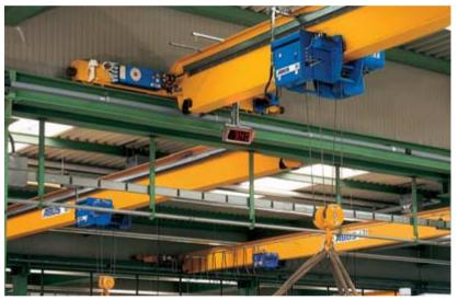
The optional large load display clearly shows the load on the hook even at a considerable distance.
