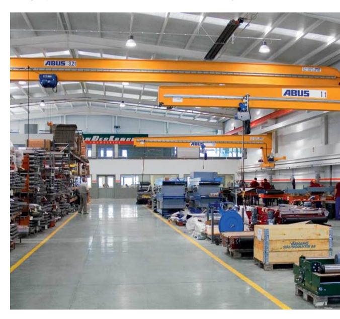
The ABUS single girder wall travelling crane is designed for operation on a lower level beneath a large travelling crane system.
