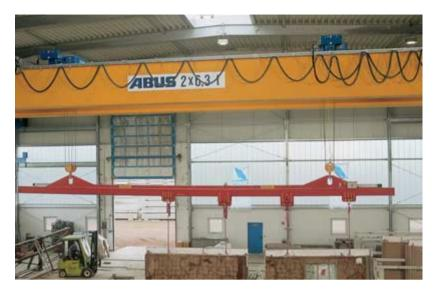
Two snychronised trolleys using spreaders ensure the reliable positioning of long loads.
