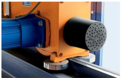
Optional: thruster rollers offer an even more exact method of crane travel guidance, reducing skewing forces.
