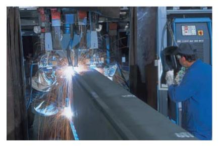
The moving portal welding unit designed in-house by ABUS personnel welds the web plates to the upper and bottom flanges and the rails on the top of the girder. The welding unit can complete up to six welds at the same time. The high-performance burners are automatically controlled by a PLC. Following the welding of the closure plates and the installation of the end carriages, the paintwork required for the specific application is applied.
