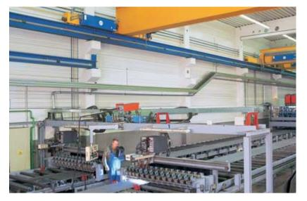
Plates of the lengths required for box girders are welded together on a PLC-controlled welding machine. The butt welding machine can process plates of different thicknesses and the automatic weld sequence control system ensures the highest welding quality possible.
