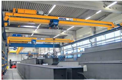
ABUS single girder travelling cranes can be equipped with identical but also with differing girder connection versions for each track. In this way, you can divide a wide factory into two sections, allowing highly flexible material handling.
