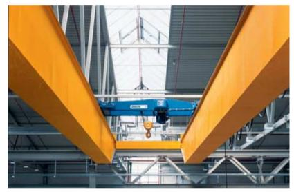
Lowered trolleys allow double-girder travelling cranes to be installed even where there is little space above the crane track. The higher position of the crane bridge with a lowered trolley may be a decisive advantage, for example when handling bulky machines or large tanks.
