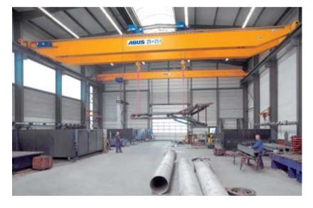
The electronic synchronisation control system allows synchronised lifting with several hoists, ensuring secure and precise load positioning at all times, even with minimal hook spacing.
