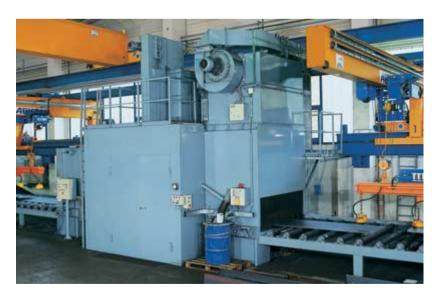
Following thorough inspection, the steel plates are derusted and descaled to ensure excellent weld quality. The shotblasting unit is equipped with four high-performance turbines and can produce surfaces to DIN 55928, Grade SA 2 ½. It can be adjusted to any steel grade and plate thickness.
