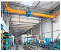
ABUS underslung travelling cranes are installed on ceiling mounted tracks rather than free standing or building columns. Advantageous side approach dimensions allow the optimum use of the entire width of the production.
