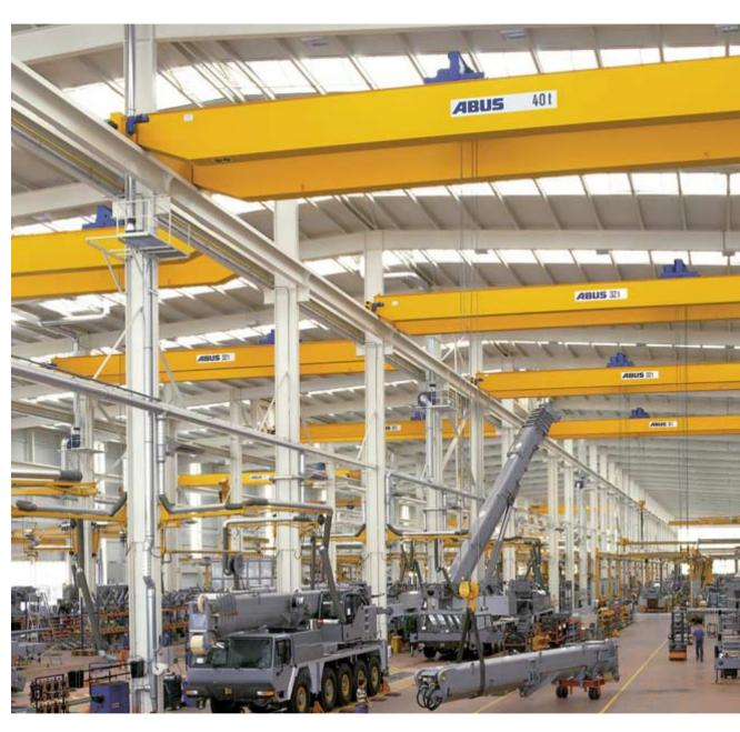
\* Details of higher load capacities and wider spans on application. Two girders are simply stronger than one, making ABUS double girder travelling cranes the ideal solution for the area coverage handling of heavy loads up to 120 t.\* Like all ABUS factory cranes, these units are available with a number of main girder connection versions to best suit new or existing buildings and the best in functionality, versatility and convenience. In addition, the
