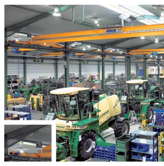
The ideal solution for a new factory: the ABUS ELK single girder travelling crane with long angle chamfer adapted to suit the building haunch (version 3), optimising available height.
