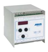
The ABUS LIS-SE load indicator system features a comprehensive range of switching and monitoring functions. The system offers an extremely short load detection time of only a few hundredths of a second, effectively protecting ABUS wire rope hoists against overloading. The measurement principle allows the load on the hoist to be limited without reducing the lifting height available.
