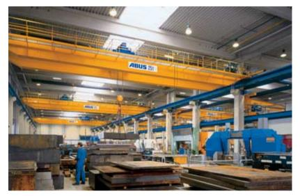
With maintenance walkways and crab unit with service platforms, all the components of the crane system are easily accessible, a crucial advantage for maintenance work.
