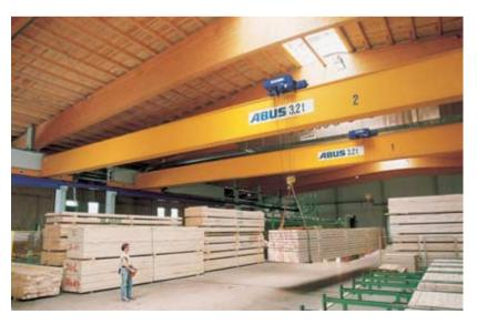
The tandem operation of travelling cranes makes it easier to handle bulky loads.
