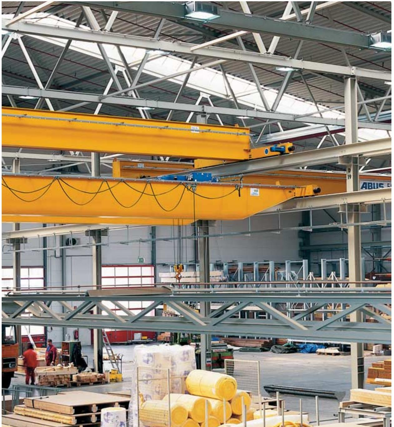
If a certain lifting height is only required in part of a hall, ABUS travelling cranes can be installed on different levels. In this example, an ABUS ELS single girder torsion box crane is used on the higher level, with an ABUS ZLK double
