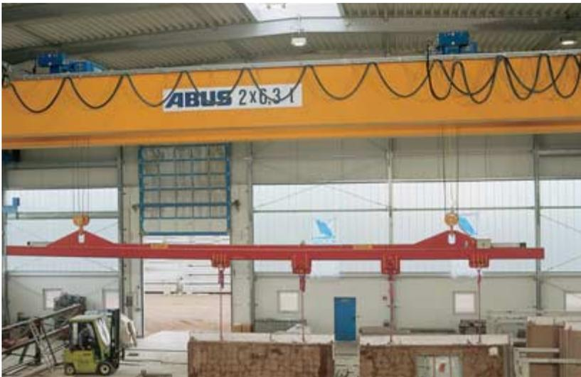
Two synchronised trolleys using spreaders ensure the reliable positioning of long loads.
