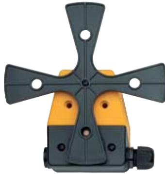
**ABUS cross-type limit switches** limit long travel and cross travel, automatically slowing or stopping the crane or the hoist at the end of the track. These limit switches may also be applied for crane zoning if it is necessary to divert a hoist on a crane around a prohibited area. The switch is operated by a switching lug installed on the crane track or on the crane bridge.
