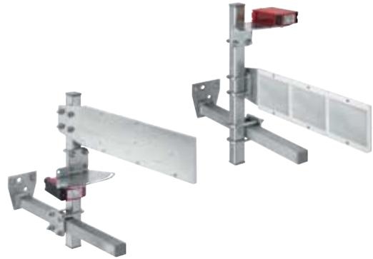
The **ABUS anti-collision device** prevents accidental collisions between cranes on the same track. The standard version slows the cranes as they approach each other. A shut-down function is optional. Special designs are also available for specific applications, such as keeping defined safety distances between two cranes.
