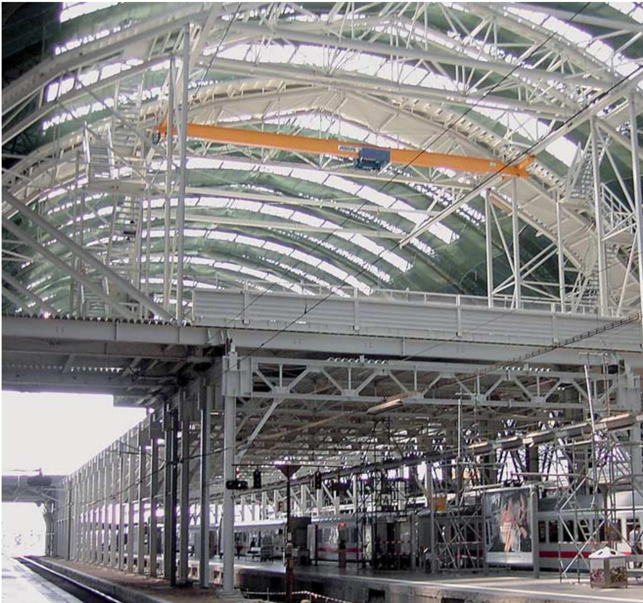
Complex factory configurations pose special problems, but they are easy to solve with ABUS underslung travelling cranes. The crane track is mounted directly on the factory ceiling and not on free standing structural or building columns, allowing efficient material handling solutions even in tight spaces with difficult design conditions.
