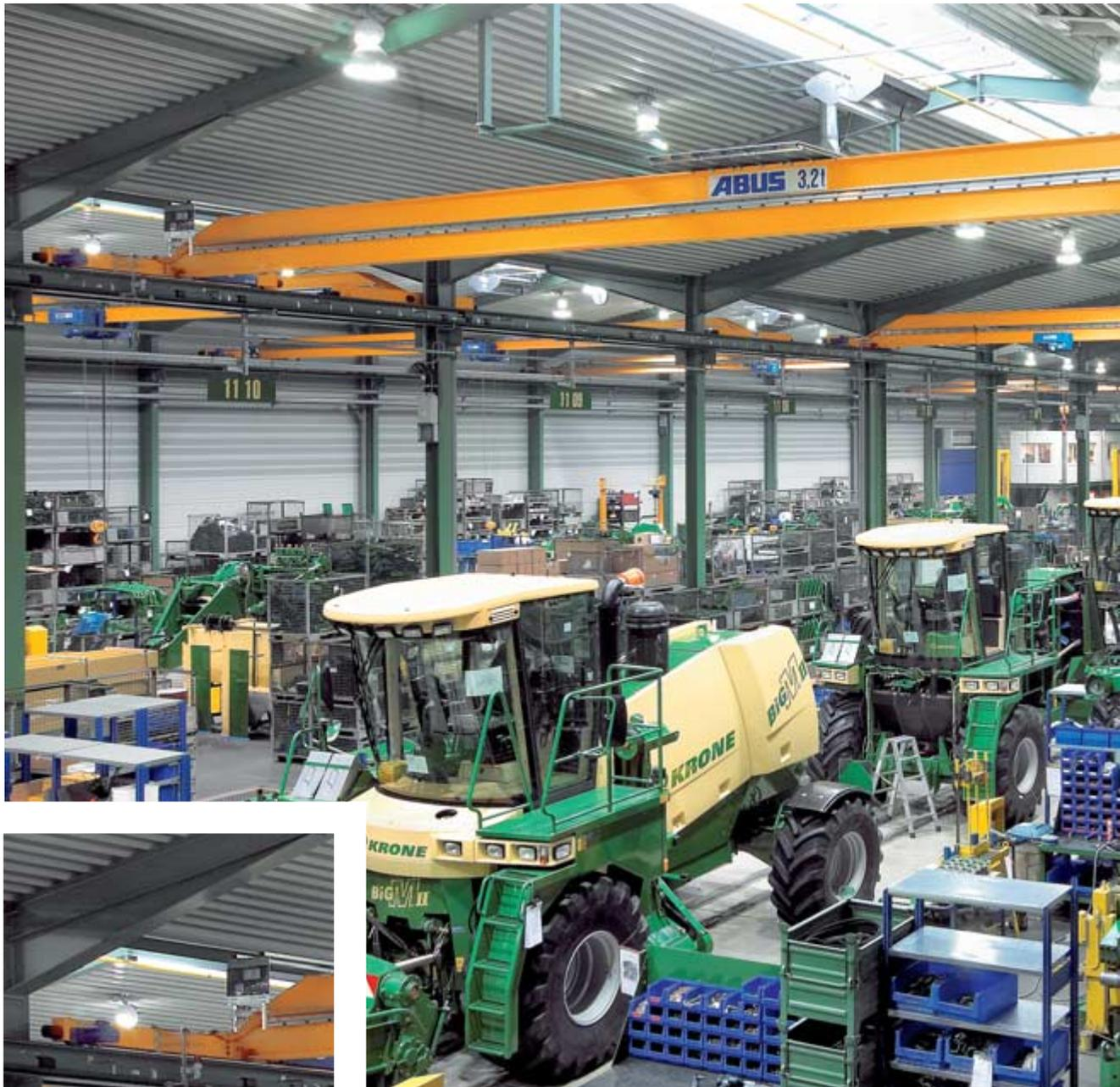
The ideal solution for a new factory: the ABUS ELK single girder travelling crane with long angle chamfer adapted to suit the building haunch (version 3), optimising available height.
