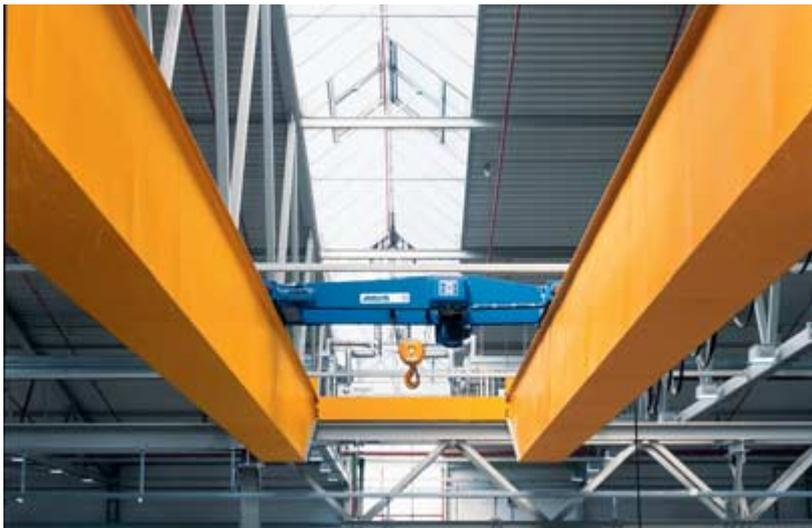
Lowered trolleys allow double-girder travelling cranes to be installed even where there is little space above the crane track. The higher position of the crane bridge with a lowered trolley may be a decisive advantage, for example when handling bulky machines or large tanks.
