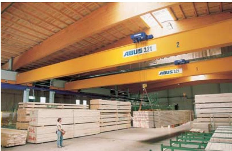
The tandem operation of travelling cranes makes it easier to handle bulky loads.
