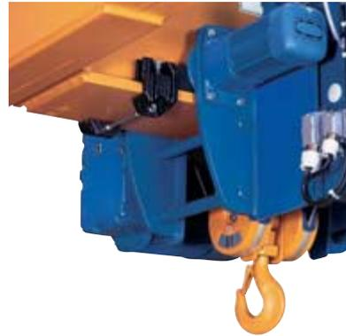
**ABUS clamping buffers** can be used for a variety of functions: for limiting crane travel, fixing hoists at specific positions, absorbing impact energy or securing trolleys against rolling away. They are adjustable and can be installed as required. In particular, they can be used temporarily, offering considerable versatility. Especially for monorail hoist trolleys, ABUS offers clamping buffers designed for adaptation to current conditions.
