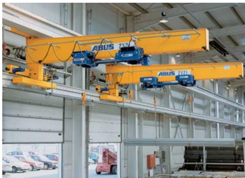
With two hoists in tandem operation, ABUS single girder wall travelling cranes can also be used for the precise positioning of long loads.
