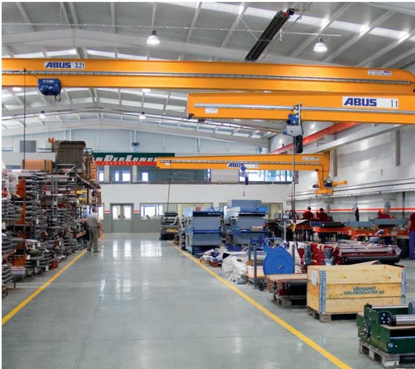
The ABUS single girder wall travelling crane is designed for operation on a lower level beneath a large travelling crane system. These cranes provide additional handling possibilities and ensure smooth and troublefree material handling between different working areas.
