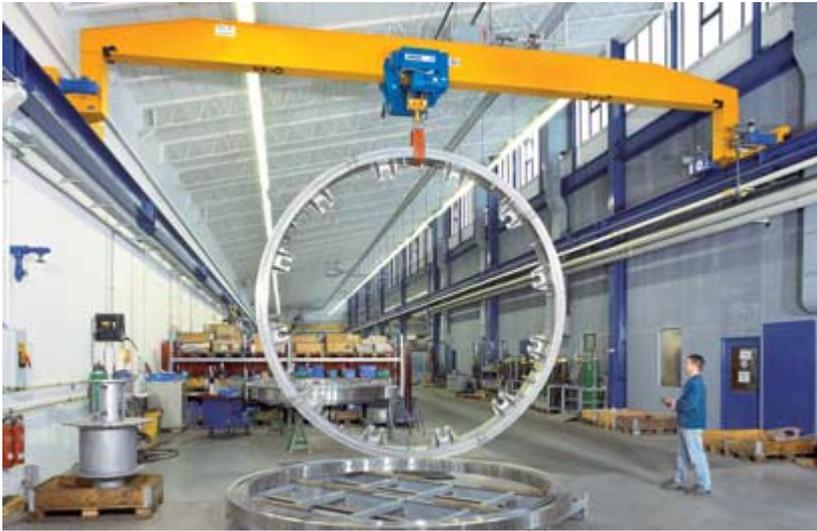
Raised-up crane bridge configurations are the ideal solution for special situations and buildings with difficult conditions.
