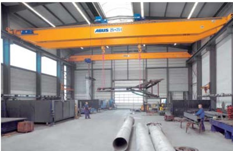
The electronic synchronisation control system allows synchronised lifting with several hoists, ensuring secure and precise load positioning at all times, even with minimal hook spacing.
