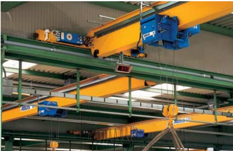
The optional large load display clearly shows the load on the hook even at a considerable distance.
