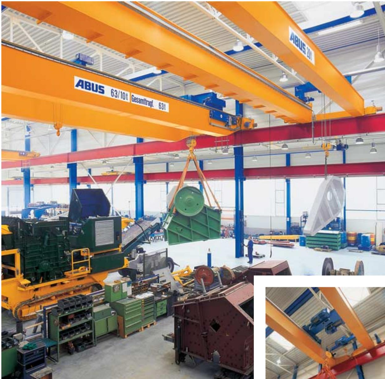
The end carriage may be mounted on eight wheels for even load distribution. Heavier loads can then be carried on a smaller crane track and the reinforcement otherwise needed in existing buildings may not be required.
