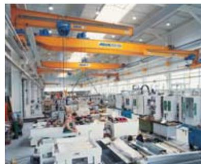
**ABUS single girder wall travelling cranes** are installed on a separate track below other types of travelling crane. They are the ideal solution for serving several working areas at the same time. The ABUS EKL single girder wall travelling crane is designed for spans up to 12 m and load capacities up to 5 tonnes.
