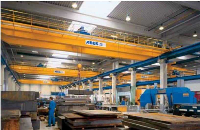
With maintenance walkways and crab unit with service platforms, all the components of the crane system are easily accessible, a crucial advantage for maintenance work.
