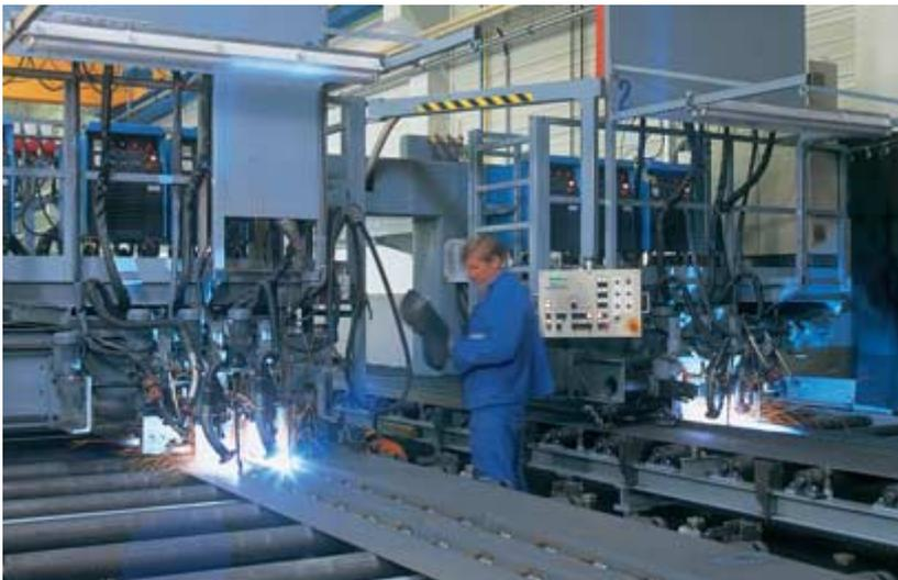
Before the next processing stage, web plates are welded into place to protect the girder against twisting; stiffeners are inserted to improve the overall stability of the structure. Following assembly on the box girder line, the box girder is ready for processing by the portal welding unit.
