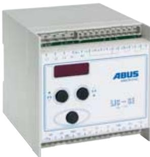
The **ABUS LIS-SE load indicator system** features a comprehensive range of switching and monitoring functions. The system offers an extremely short load detection time of only a few hundredths of a second, effectively protecting ABUS wire rope hoists against overloading. The measurement principle allows the load on the hoist to be limited without reducing the lifting height available.
