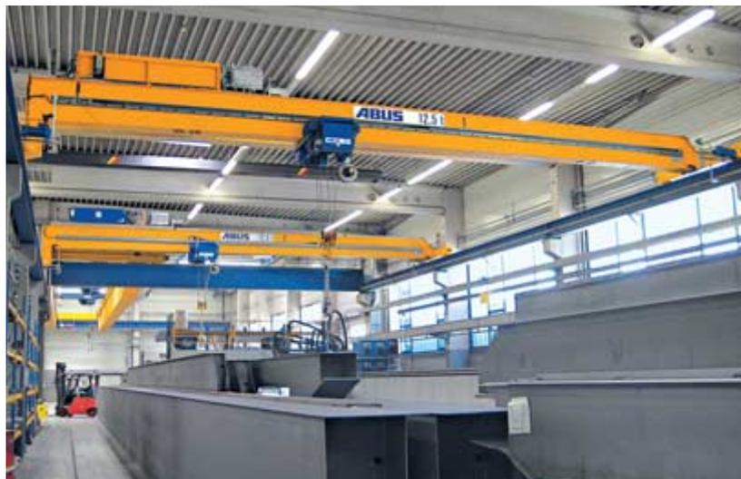
ABUS single girder travelling cranes can be equipped with identical but also with differing girder connection versions for each track. In this way, you can divide a wide factory into two sections, allowing highly flexible material handling.
