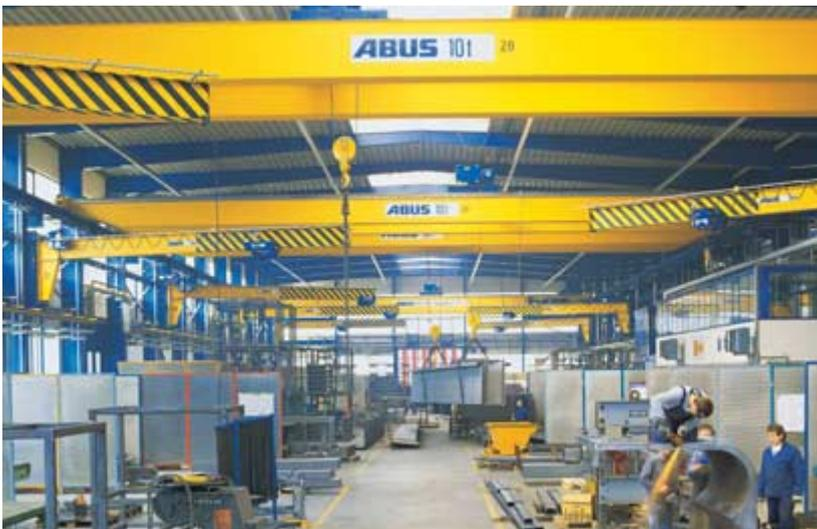
ABUS two fall wire rope hoists are designed for high lifting speeds and load capacities up to 20 t. In this example, wall-mounted jib cranes provide flexible material handling on the lower level.
