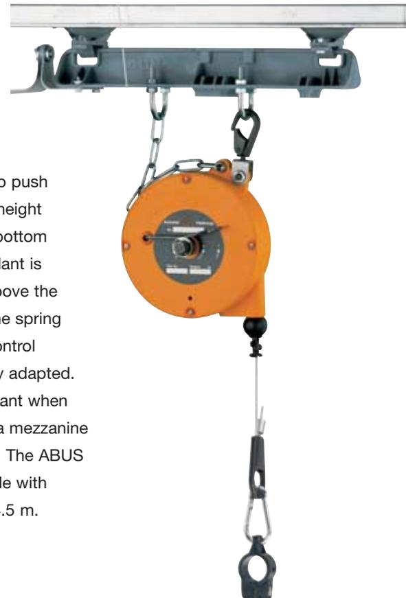
**ABUS spring reels** keep push button pendants at the height required. Normally, the bottom of the push button pendant is positioned one metre above the operating level. Using the spring reel, the length of the control cable can be individually adapted. This is especially important when operating a crane from a mezzanine floor or an assembly pit. The ABUS spring-reels are available with cable lengths of 3 and 4.5 m.
