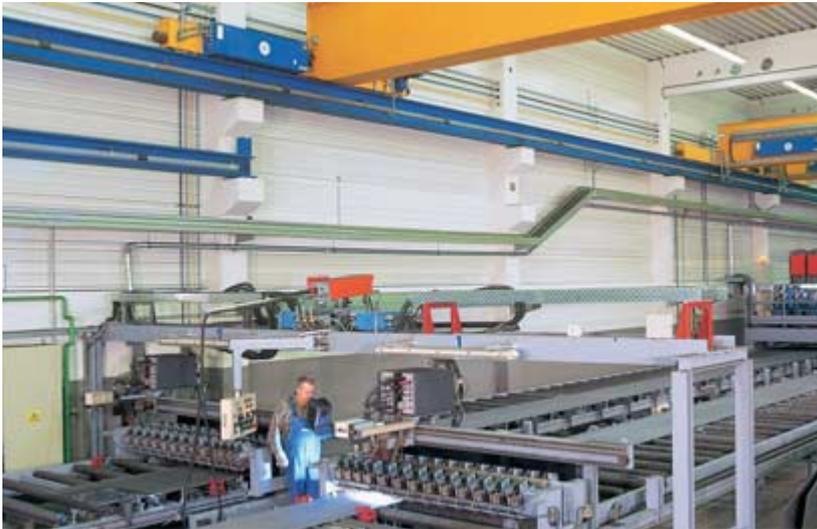
Plates of the lengths required for box girders are welded together on a PLC-controlled welding machine. The butt welding machine can process plates of different thicknesses and the automatic weld sequence control system ensures the highest welding quality possible.
