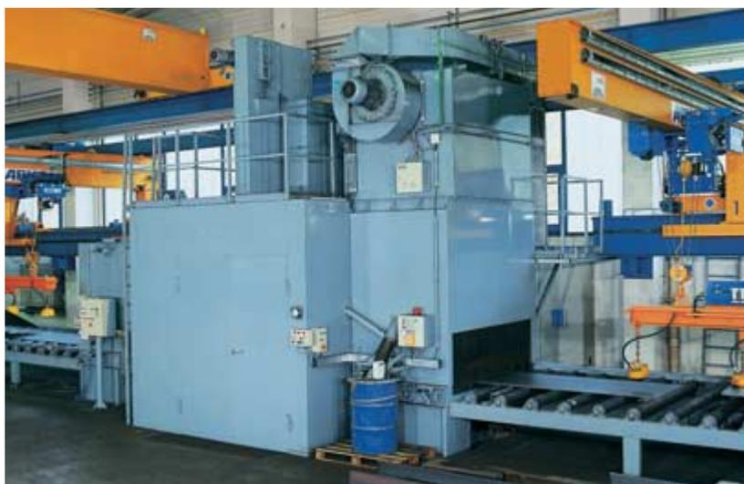
Following thorough inspection, the steel plates are derusted and descaled to ensure excellent weld quality. The shotblasting unit is equipped with four high-performance turbines and can produce surfaces to DIN 55928, Grade SA 2 ½. It can be adjusted to any steel grade and plate thickness.
