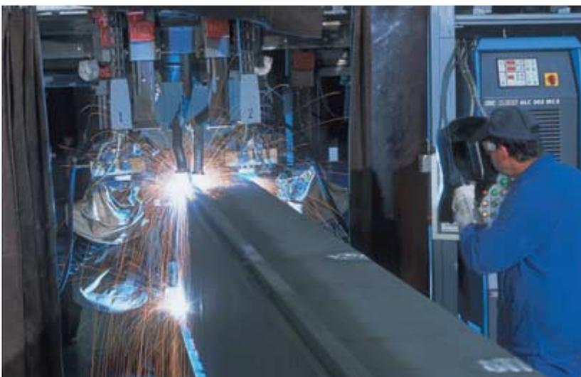
The moving portal welding unit designed in-house by ABUS personnel welds the web plates to the upper and bottom flanges and the rails on the top of the girder. The welding unit can complete up to six welds at the same time. The high-performance burners are automatically controlled by a PLC. Following the welding of the closure plates and the installation of the end carriages, the paintwork required for the specific application is applied.
