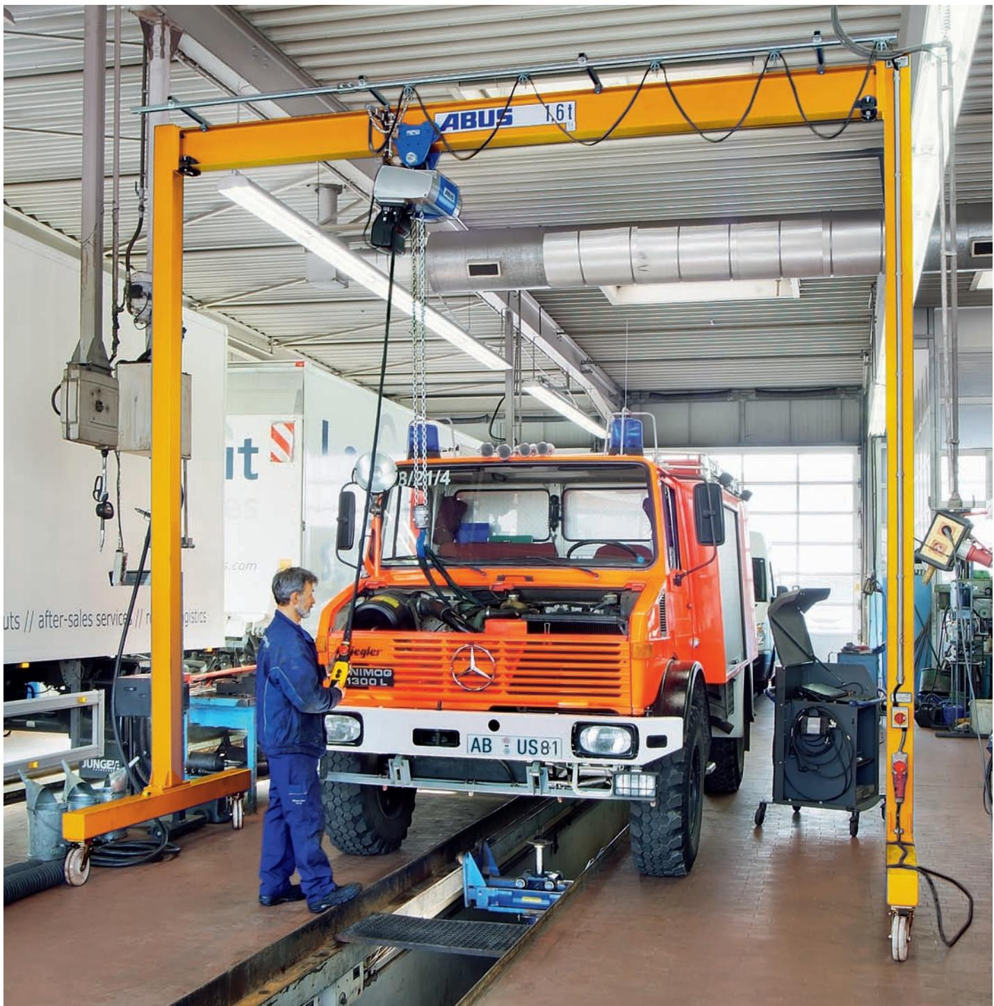
The ABUS LPK mobile gantry is the right solution if a permanently installed hoist is not needed but crane usage is required at several different points. The crane is designed for ABUS electric chain hoists with load capacities up to 2000 kg.
